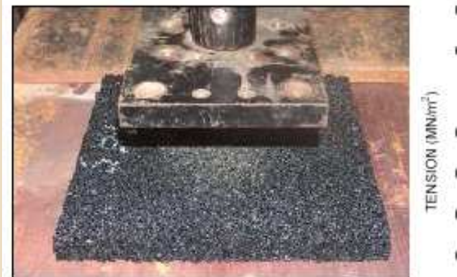
Secant static stiffness test (up) & Dynamic stiffness test (down)
